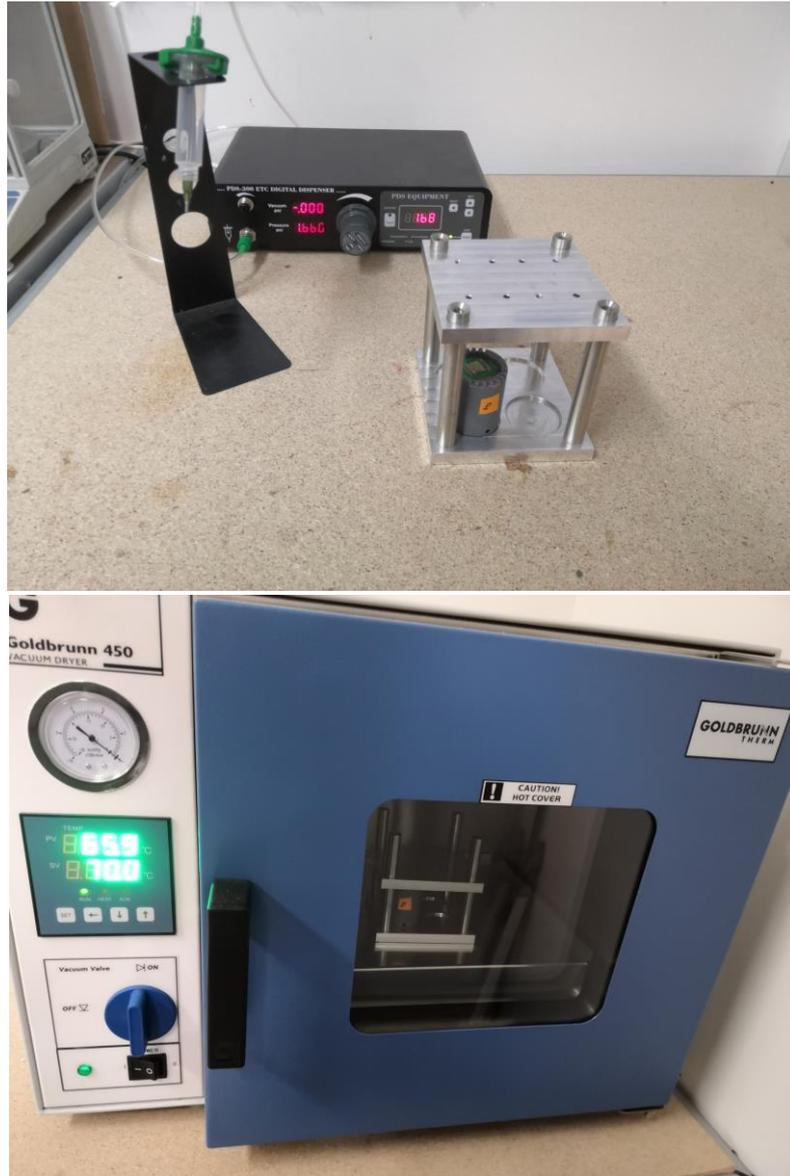
Figure 30: Top: the glue dispenser and Head holding mechanism with a LOTUS head, Bottom: Head holding mechanism with a LOTUS head in the oven
