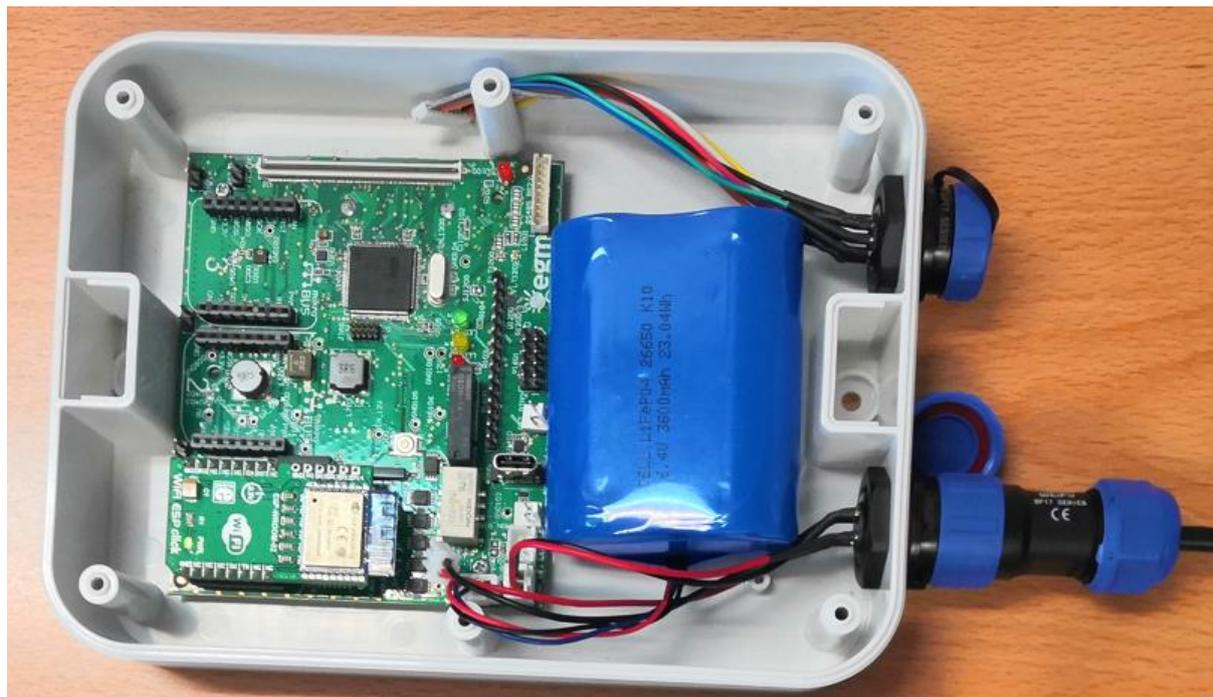
Figure 4: The LOTUS box with its electronic cards and cell batteries
